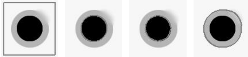
Figure 1.17: Strong neighbouring edge leakage - from left: initial snake, geodesic snake steps through weak edge in top right of outer boundary, GGVF is attracted by the stronger inner edge, RAGS snake converges properly using extra region force.
