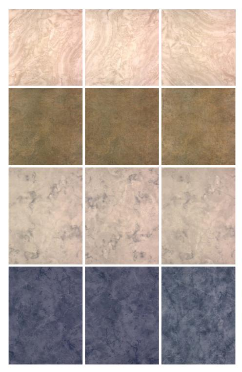
**Figure 3.1:** Colour shade examples from the COLSHADE dataset - left column: tile images with standard normal colour shade; middle column: tile images with minor colour shade problem; right column: tiles with relatively larger colour shade off-set.
