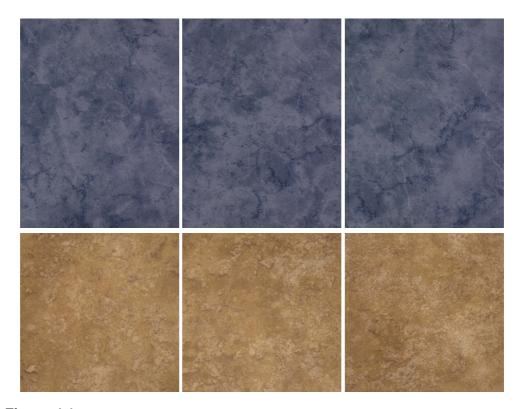
**Figure 4.1:** Two examples of ceramic tiles with different colour shades from dataset COLSHADE - from left: The first two images in each row belong to the same colour shade, the last one in each row is an example of off-shade.
