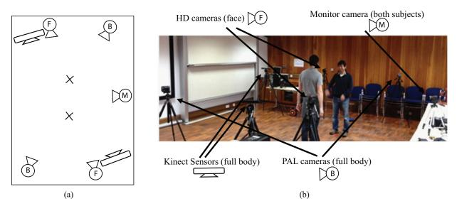
Fig. 1. CONVERSE data capture environment. a) Plan view of the capture setup b) Photo of subjects in situ.
