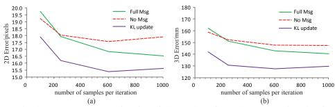
Figure 5: The average error as a function of the number of samples used per iteration for the 2D reprojection error (a) and 3D reconstruction error (b). Full Msg and No Msg show the error without the KL divergence method with and without message passing. KL update shows the error using the KL divergence update method with message passing.
