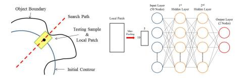
**Fig. 2.** Left: Schematic diagram of local patch intensity extraction. Right: Example NN architecture with 2 hidden layers.
