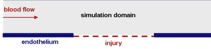
Figure 1: Schematic representation of a 2D vessel for the simulations: the reactive wall is a part of the lower wall. Symmetry of the geometry is assumed.
