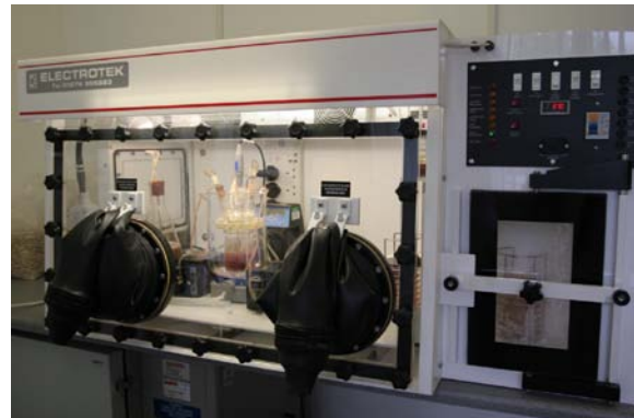
Figure 2 The in vitro fermentation model
