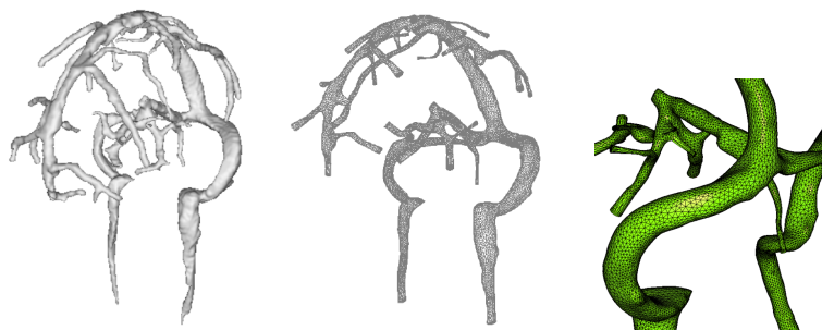
Figure 2: One example of a vascular model (left), of the 3D corresponding tetrahedral mesh of 237438 elements (middle), magnified view of the mesh (right).
