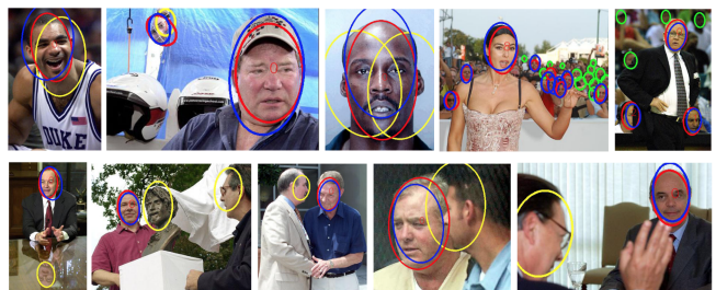
Fig. 6. First row: examples of false positives and false negatives. Second row: examples of correct detections but counted as false positives. (red: ground truth, blue: true positive detection, yellow: false positive detection, green: false negatives).
